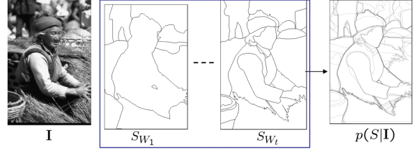
Figure 1. Manual segmentations of an example image and the corresponding edge maps. For illustration purpose, we show the negative of the probability so the darker the pixel, the higher the probability of an edge.
