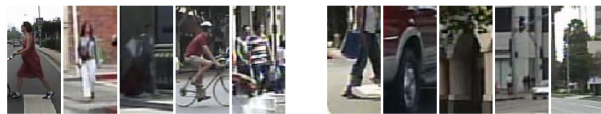
Figure 10. Selected HOG false negatives (left) and high confidence false positives (right) for near scale unoccluded pedestrians.
